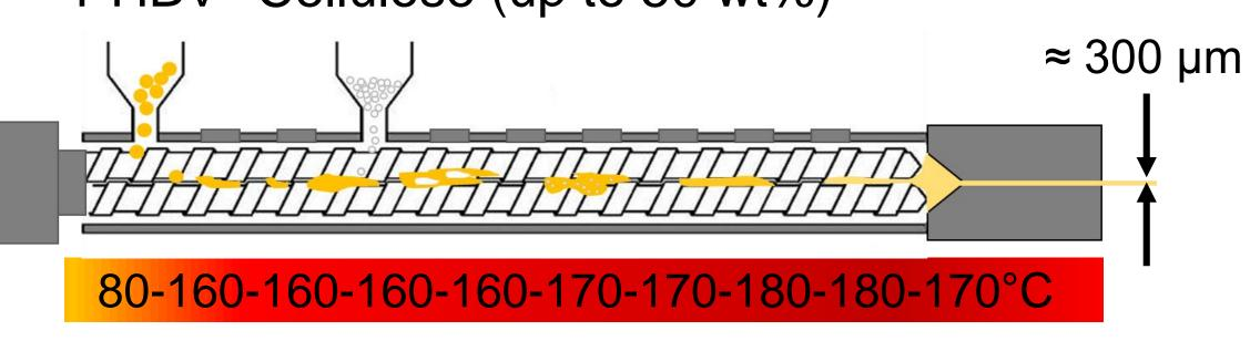
Scheme of the twin-screw extruder with the temperature profile.
