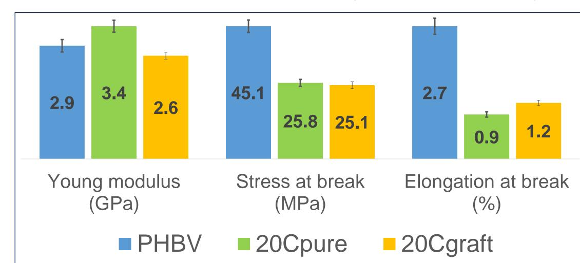
In both cases, adding particles weakens the biopolymers. Grafting of cellulosic particles makes the composite slightly more ductible than the classic one, so more processable. The stress at break is not improved as expected.
